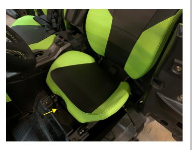
• Remove two 12mm bolts on front of drivers seat
