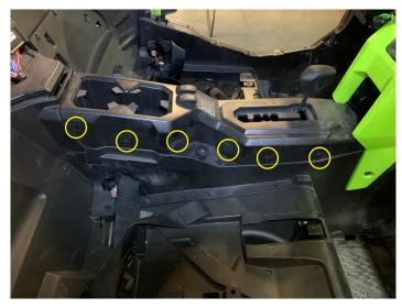
• Remove the five push pins on the driver side console on the passenger side
