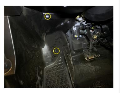
• Remove two 5mm allen bolts from behind glove box door
