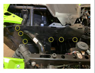
Install four 10mm bolts, four push pins and five 5mm allen bolts to remove top of dash
