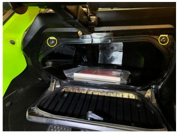
• Install the bottom steering wheel cover
