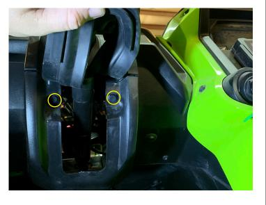
• Reposition bottom half of the steering colum rubber boot
