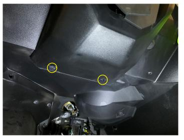
• Remove the bottom steering wheel cover
