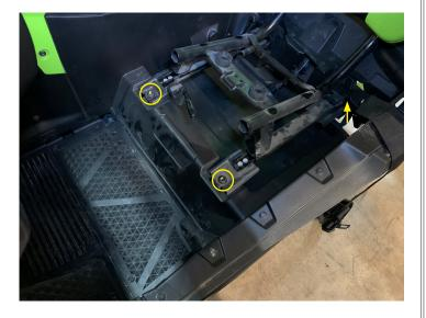
• Release latch at front of driver and passanger lower cushions to install
