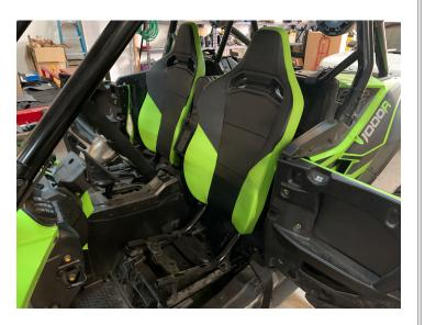
• Remove two push pins on front of passenger seat and then remove the covers
