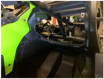
• Remove one 5 mm allen bolt and one push pin from passenger kick area
