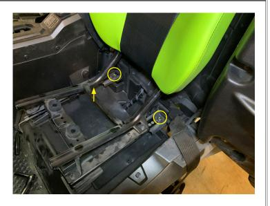
Install two 12mm bolts on front of drivers seat
