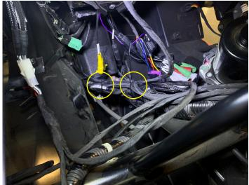
Install power harness to each amplifier (Connector with bullets connects to NA2-400.2)
