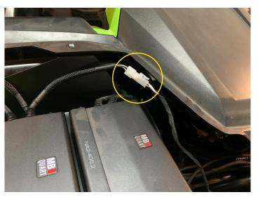
• Route subwoofer and rear speaker harness down toward center console going to the rear of the vehicle. (Stage 3 does not include rear speakers but run harness for easy upgrade in the future)
