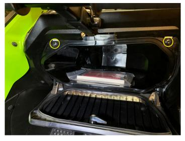
• Remove one push pin in the back of the glove box
