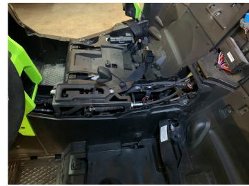
Install the five push pins on the driver side console like on the
