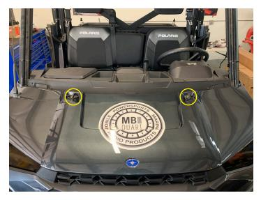
• Remove two push pins from center cup holder
