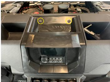
• Place center console in the vehicle sliding forward then down
