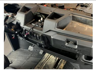
• Install three push pins on driver side of dash
