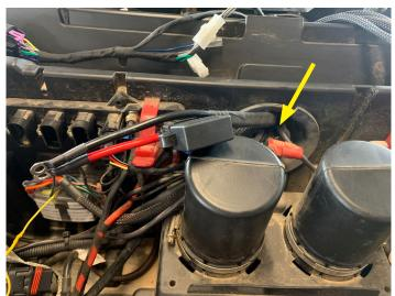
Connect the power and ground wires by removing the 10mm nuts on the pulse junction block
