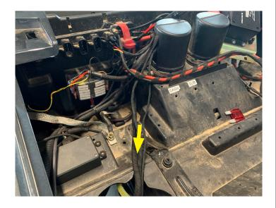
Pass the wiring around any moving parts and down the frame toward the center console and secure in place with zip ties
