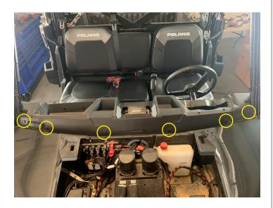
• Lift up on the dash and remove from vehicle
