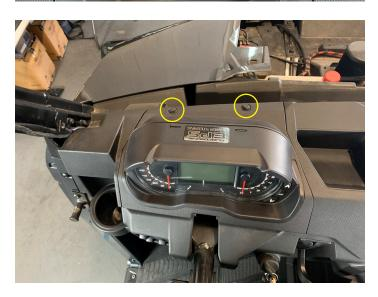
Open upper glove box and remove four T20 torx screws and then lift assembly out of vehicle
