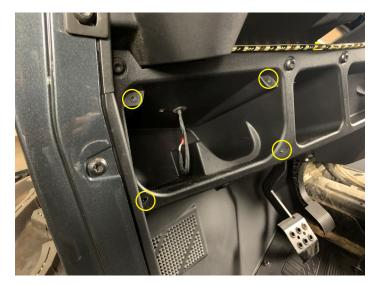
Connect the speaker wires to the speaker and then install the speaker and grill assembly with four high-low Torx screws and washers using a T25 Torx bit
