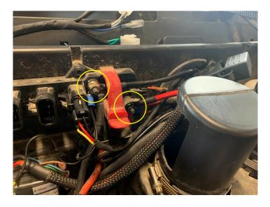
Connect the blue wire from the amplifier harness to the blue wire on the radio harness
