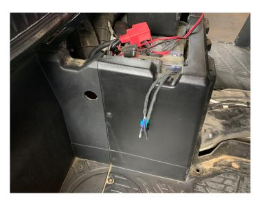
Drill ??" hole and pass subwoofer connection through hole and place grommet
