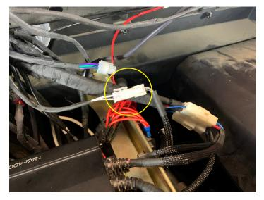
Connect the speaker y-harness to the front and rear speaker harnesses
