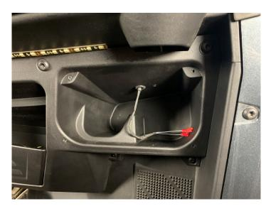
On the radio harness pass the power connection through the grommet toward the front of the vehicle and plug into an open port on the pulse junction block
