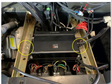
• Plug in the amplifier harness connectors to the amplifiers
