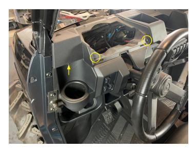
• Remove six push pins from the front of the dash
