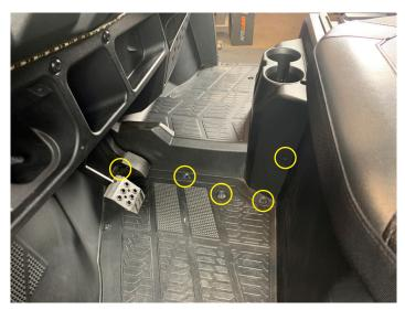
Lift center console upward starting at cupholder and remove from vehicle
