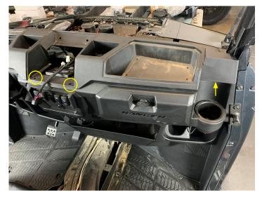
• Install upper glove box with four T20 Torx screws
