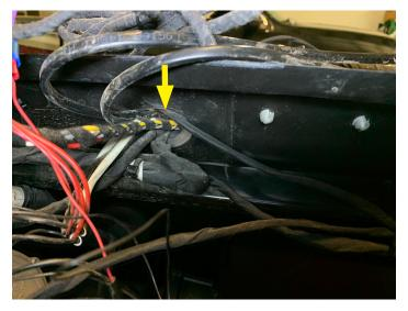
• Route rear wires out grommet toward under hood area as seen by arrow (May need to reach from inside console area)
