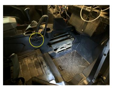
• Install center cover with two push pins
