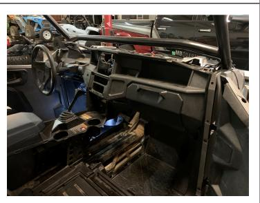
• Connect speaker wires and then hold passenger side pod up high to the dash till it slides into place and using 11/32" drill bit, drill the four holes and secure with four push pins
