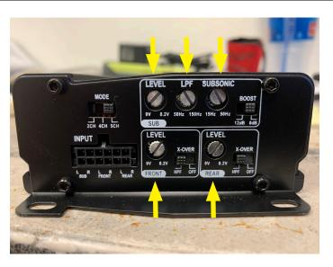
Use four M3 Philips screws to secure amplifier to plate and position gain / crossover facing toward center of vehicle
