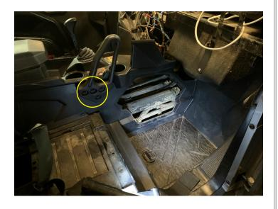
• Remove six push pins and three T40 bolts
