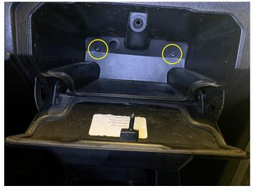
• Install instrument cluster with two 10mm bolts
