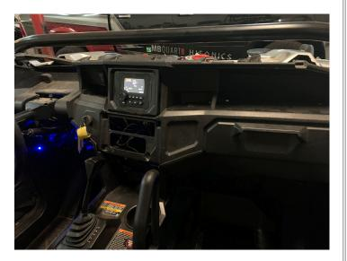
Install key switch and align to detent
