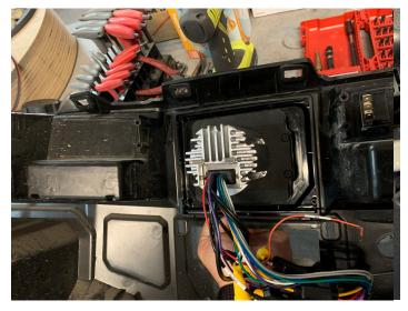
• Position rear bracket and loosely install the two nuts on back of radio
