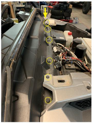
Remove top two push pins from driver and passenger door opening
