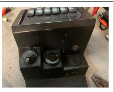
• Install the USB / AUX port in this hole (PASP-18)
