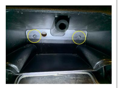
• Remove two T40 bolts in front of the shift knob
