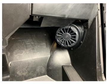
• Repeat Step 2 on the driver side and drill the five lower holes with 11/32" drill bit and secure with five push pins
