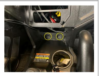
Install two T40 bolts in passenger glove box
