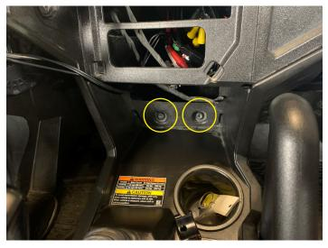
• Remove two T40 bolts from inside the glove box
