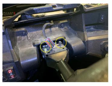
Install two T40 bolts in center console
