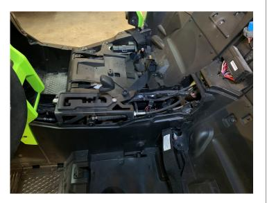
• Install the five push pins on the driver side console like on the passenger side
