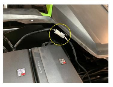
Route subwoofer and rear speaker harnesses down toward center console going to the rear of the vehicle
