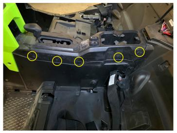
• Place gear selector to "H" and remove the top of the center console
