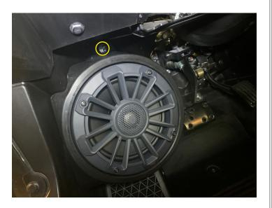
• Tighten the 5/16" bolt in the fender area
