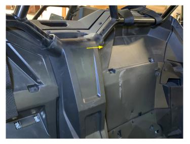
• Using a small flat head screwdriver push in the center and remove the six clips on the passenger side
