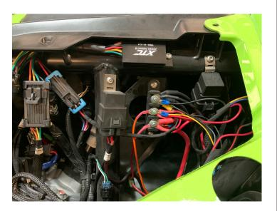
• Plug RCA into the NA2-400.2 and run to the front RCA outputs of the radio
