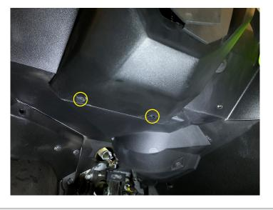
• Remove the bottom steering wheel cover
