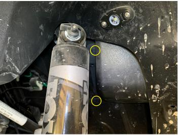
• Pull down or remove air intake cover
