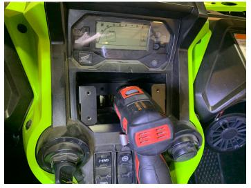
• Install two 5mm allen bolts through the bracket and pocket and install a flat washer and lock nut (You may need to ask a friend for help or can reach on both sides of the dash to tighten)
