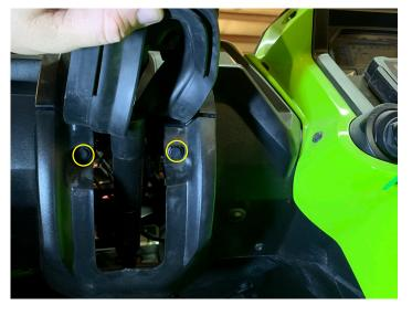
• Reposition bottom half of the steering column rubber boot
