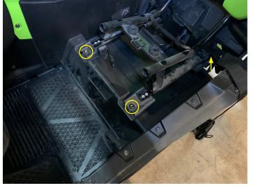
• Slide driver seat forward and remove two 12mm bolts on rear of seat
