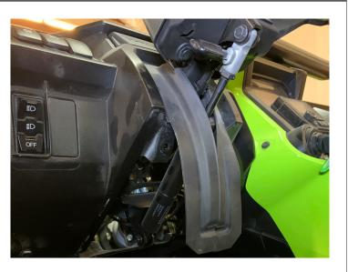
• Remove one 5mm allen bolt and one push pin from the drivers kick area
