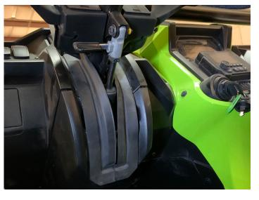
• Place gear selector to "H" and install the top of the center console
