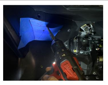
• Pass the wire from the driver side pod through the hole you drilled
