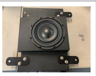
• Place subwoofer enclosure under driver seat area and pass the harness through small opening pictured and pull toward top of center console
