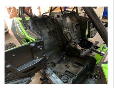
• Pull top fuse access panel toward front of vehicle and remove
