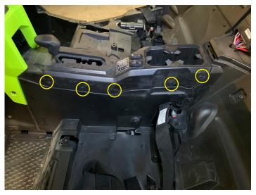
• Using a small flat head screwdriver push in the center and install the six clips on the passenger side
