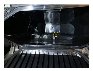
• Remove three push pins from below the glove box
