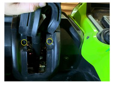
• Remove the two push pins on the bottom of steering column cover
