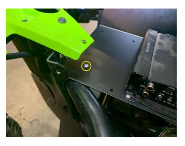
Install the NA2-400.1 amplifier next to the two channel amplifier and secure with three M4 Philips screws, washers, and lock nuts
