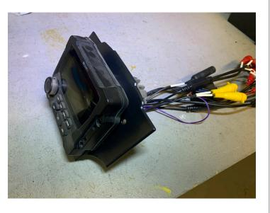
• Pass the wires from the radio through the hole below the u-bracket in the pocket
