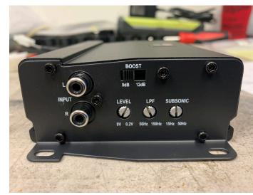
• Connect the speaker harness to the NA2-400.2 amplifier and route the driver and passenger speaker leads to the appropriate kick area
