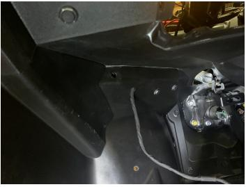
• Position pod and lightly thread a 5/16" bolt and washer from the front fender area into the threaded insert on the back of the pod
