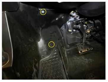
• Remove two 5mm allen bolts from behind glove box door
