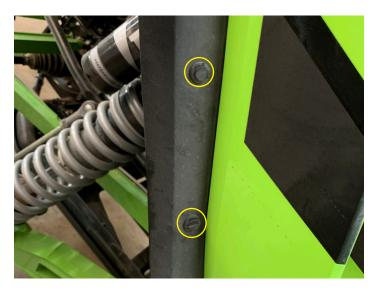
• Remove two push pins behind the passenger rear shock
