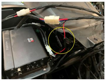
• Connect Delphi connector on power harness into the radio harness
