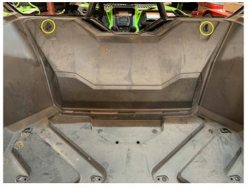
• Install three push pins from below the glove box
