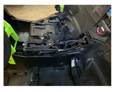
• Lift up the bottom half of the steering column rubber boot
