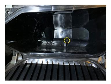
• Install two 5mm allen bolts from behind glove box door
