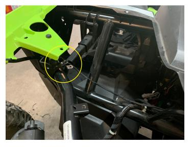
• Slide the top amplifier mount between the frame and top of dash as pictured
