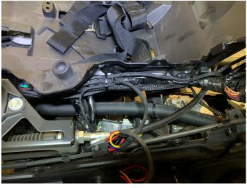
• Pass the wires through the rear firewall and upward between airbox and firewall
