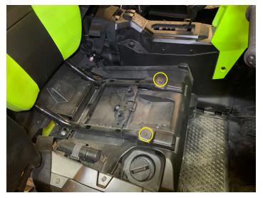
• Remove two 12mm bolts and two 12mm nuts on the passenger seat base
