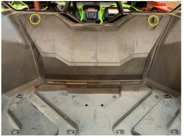
• Remove the air intake cover from the passenger rear fender area by removing ten push pins (Each location to follow)
