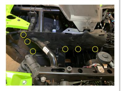
• Install four 10mm bolts, four push pins, and five 5mm allen bolts to remove top of dash
