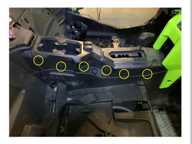
• Remove the five push pins on the driver side console like on the passenger side
