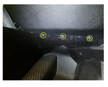
• Install one push pin in the back of the glove box
