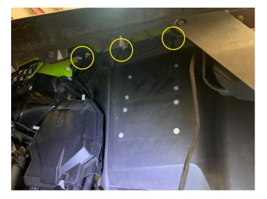
• Drill <sup>1</sup>/<sub>2</sub>" hole on either side of the bed area as shown
