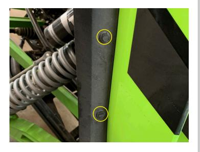
Install three push pins from inner lip of fender
