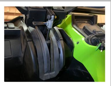
• Remove the two push pins behind the rubber boot
