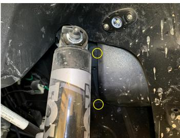
Install two push pins behind the passenger rear shock
