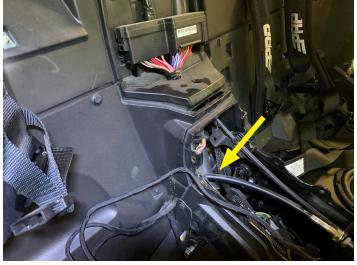
• Follow OEM wiring on each side zip tieing speaker harnesses moving toward tail lights
