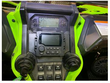
• Install four M4 cap head bolts through the face of the radio and dash into the u-bracket and tighten
