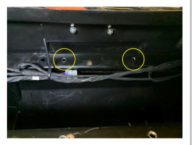
Rotate enclosure toward bracket lifting upward and using a 4mm allen wrench loosely install the three M5 button head bolts with thread patch to the top of the enclosure
