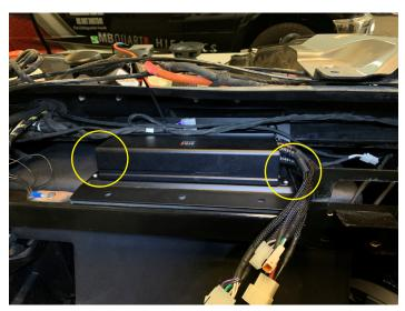
Connect Power, Subwoofer, Speaker, and RCA pigtail connectors (Note – Bass knob can be connected if wanted but the GMR-LED has subwoofer level control)
