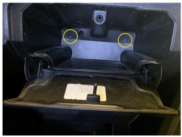
Install instrument cluster with two 10mm bolts
