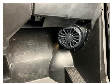
Repeat Step 2 on the driver side and drill the five lower holes with 11/32" drill bit and secure with five push pins
