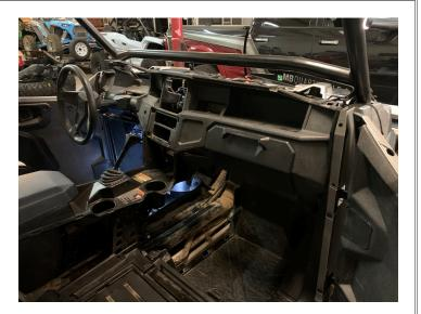
Connect speaker wires and then hold passenger side pod up high to the dash till it slides into place and using 11/32" drill bit, drill the four holes and secure with four push pins
