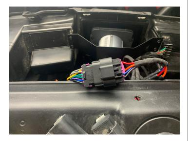
Connect the RCA input from the amplifier to the RCA output of the radio with the three 6" RCAs.
