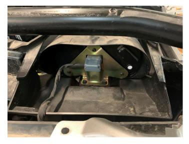
Connect switches, 12-volt accessory port, and connect USB / AUX port to radio then snap center section to dash
