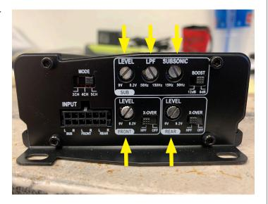
Use four M3 Philips screws to secure amplifier to plate and position gain / crossover facing toward center of vehicle
