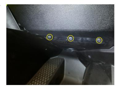
• Install one push pin in the back of the glove box
