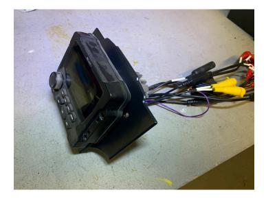
Pass the wires from the radio through the hole below the u-bracket in the pocket
