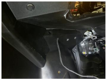
Position pod and lightly thread a 5/16" bolt and washer from the front fender area into the threaded insert on the back of the pod
