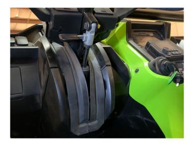
• Remove the two push pins behind the rubber boot
