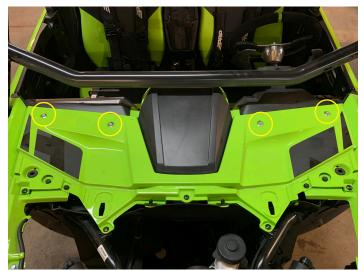
• Remove half mud guard with six push pins
