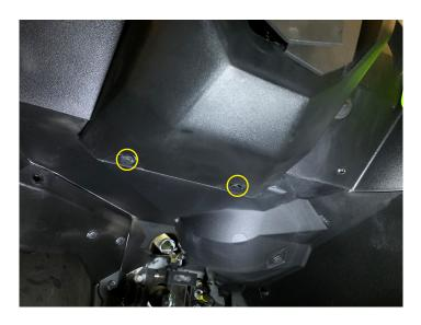
• Remove the bottom steering wheel cover
