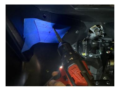
• Pass the wire from the driver side pod through the hole you drilled
