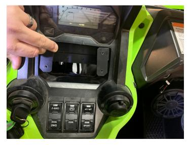
• Drill two ¼" holes using the u-bracket as a guide in the back of the pocket
