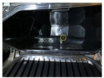
• Install two 5mm allen bolts from behind glove box door
